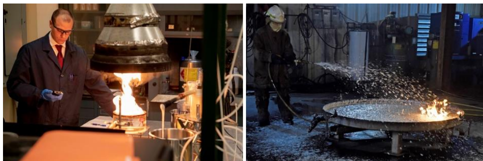
Naval Research Lab Research Chemist Spencer Giles (left) prepares to test an experimental aqueous film-forming foam at the NRL in Washington, Sept. 23, 2019. John Farley, director of fire test operations at the Naval Research Laboratory, (right) tests the effectiveness of aqueous film-forming foam by spraying it on a gasoline fire at the laboratory in Chesapeake Beach, Md. Oct. 25, 2019
